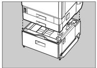
Take out the packaged items, making sure there are two thumb screws and one mounting bracket. Close the tray of the 2000-sheet large capacity tray firmly.
